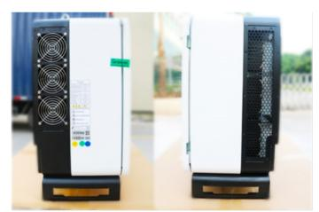
From the side view of the inverter, we can tell that the inverter is designed with fan cooling with horizontal air duct, where the air comes in from left side and goes out from the right side. Its three external cooling fans will ensure that the inverter won't be derated under high temperature conditions.
