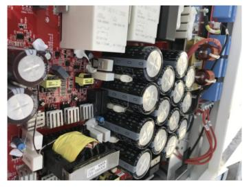
This inverter electrolytic capacitor brand is Nichicon from Japan, and the thinfilm capacitor uses the VISHAY brand from the US. The specification design strictly refers to the 1100Vdc. For example, the electrolytic capacitor is 550V for series connection.
