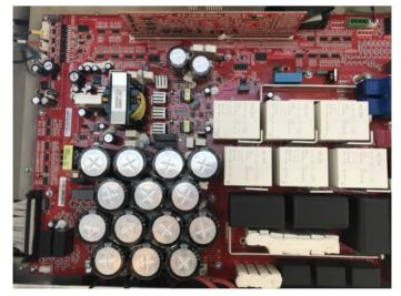
To evaluate whether an inverter is reliable, the first thing is to look at its design, and then look at its materials. The material used in this inverter is also very well-known. It is said that the most influential device inside the inverter is the capacitor. The bus capacitor of this inverter used the design method of combination of electrolytic capacitor and film capacitor. I also know that the first-tier brand inverters such as Huawei use this design.
